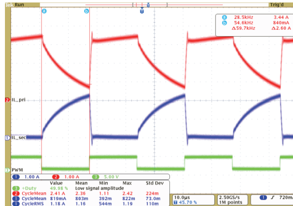
Fig. 14. Waveforms from DC-DC BF system operation with resistance load: 1 – diode D2 current(1 A/div), 2 – input current (1 A/div), 3 – PWM signal (1 A/div)
