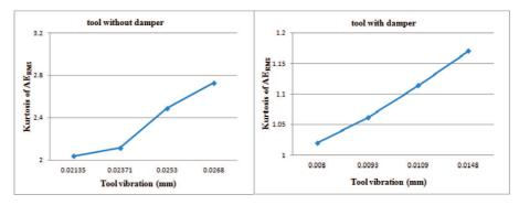
Fig. 10. Kurtosis of AE<sub>RMS</sub> vs. amplitude of tool vibration
