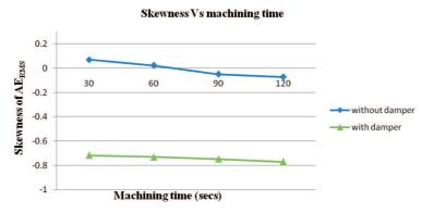
Fig. 9. Skewness of AE<sub>RMS</sub> vs. machining time
