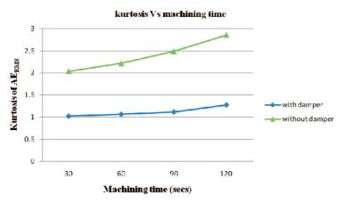
Fig. 8. Kurtosis of AE<sub>RMS</sub> vs. machining time
