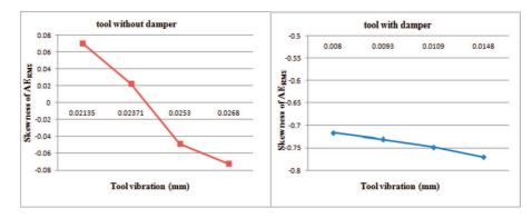
Fig. 11. Skewness of AE<sub>RMS</sub> vs. amplitude of tool vibration
