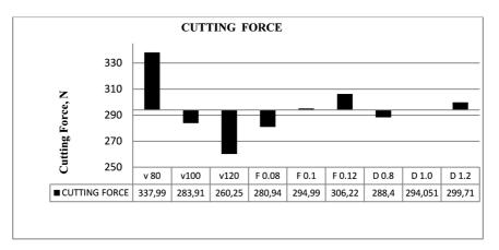
Fig. 5. Relative significance of input parameters on cutting force
