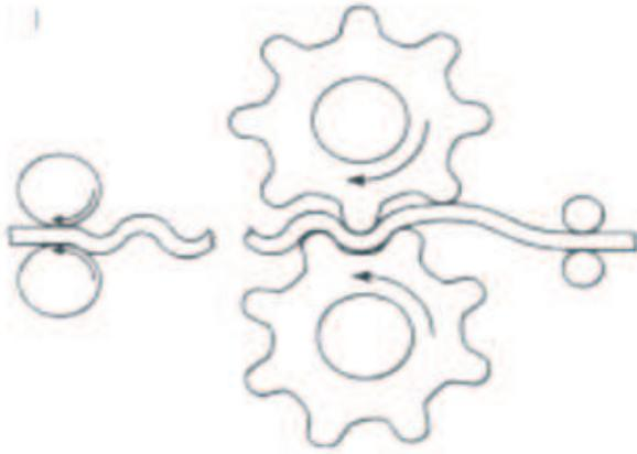
Fig. 1. Scheme of continuous RCS method [17]
