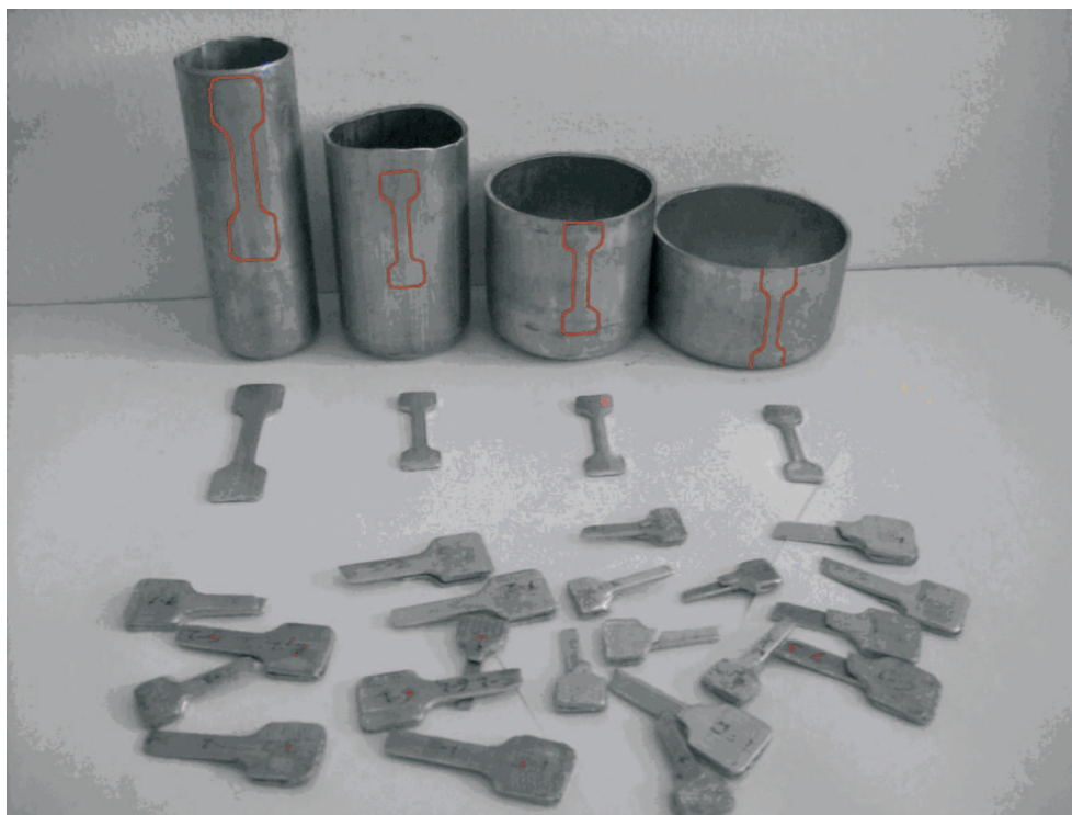
Fig. 5. Cutting out places of tensile test specimens
