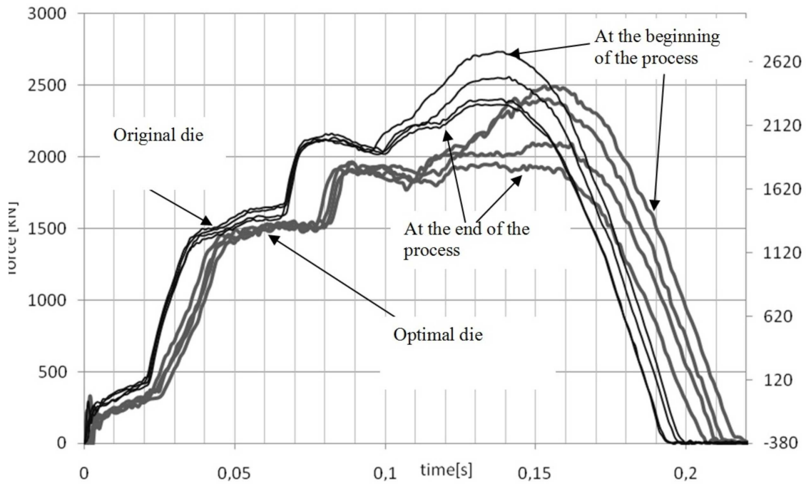
Fig. 12. Force versus time graphs for original die and optimized die in real processes
