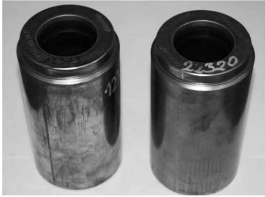
Fig. 10. Optimized tools for forging CVJ casing
