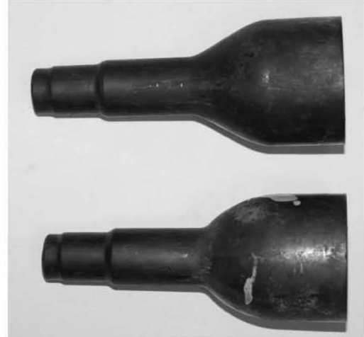
Fig. 11. Shapes of forgings obtained a) after optimization, b) before optimization
