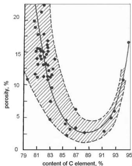
Fig. 5. Changes in porosity of hard coals versus metamorphism stage (Kawęcka 1988)
