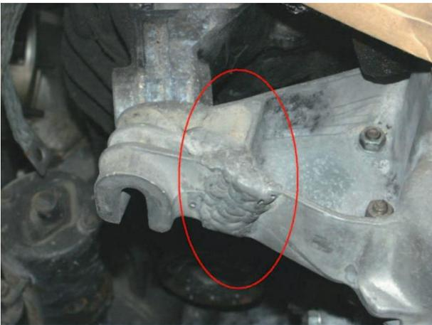
Fig. 1. Magnesium weld sample of a 914 Porsche gearbox
