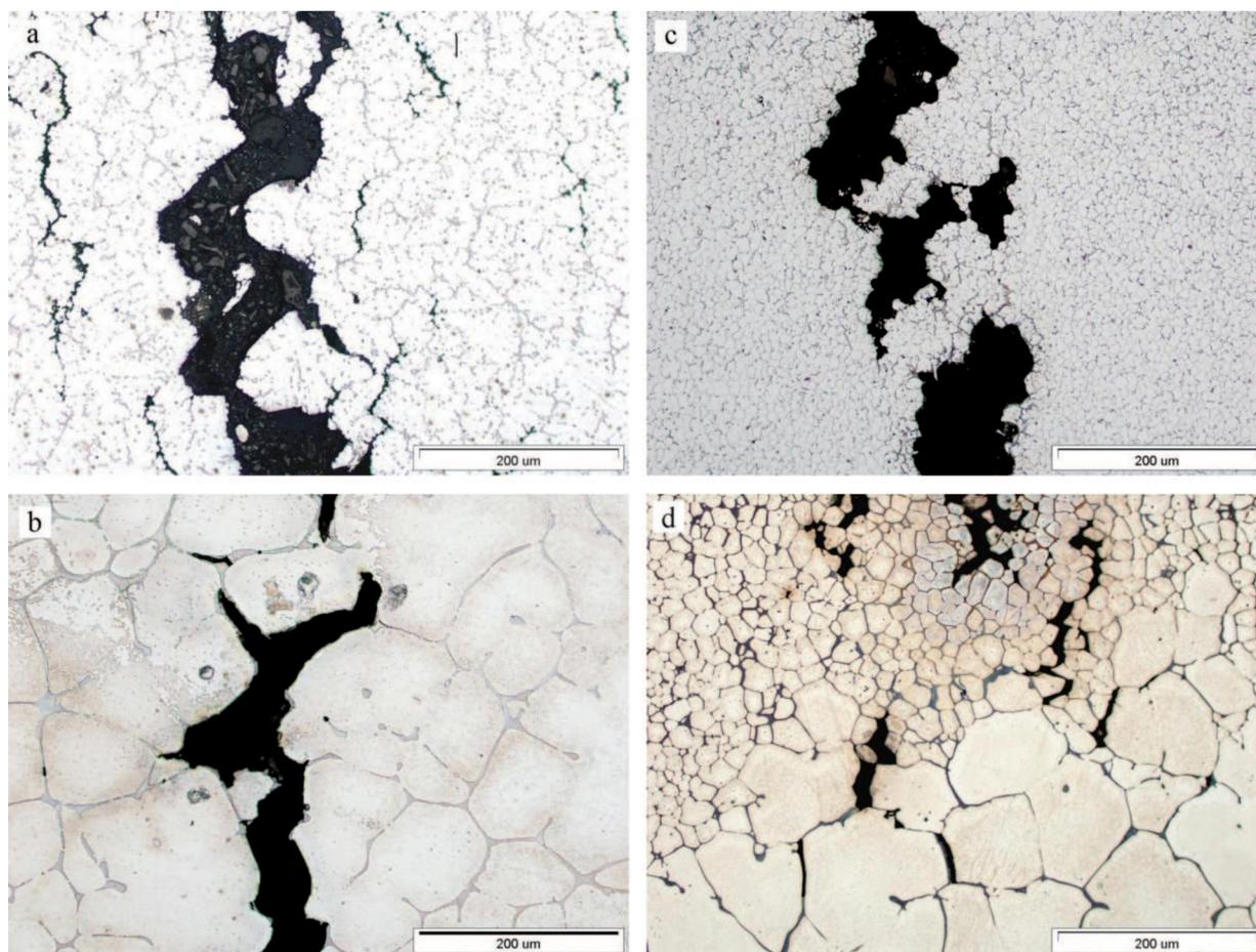
Fig. 8. Hot cracks in magnesium alloy after Houldcroft test, delivery state: a) a hot crack with visible bridges in AZ91, b) the crack with precipitations of  $(Mg,Zn)_{12}RE$  phase in ZRE1, c) a hot crack with visible bridges in WE43, d) a net of hot cracks on the melt-down line in MSRB
