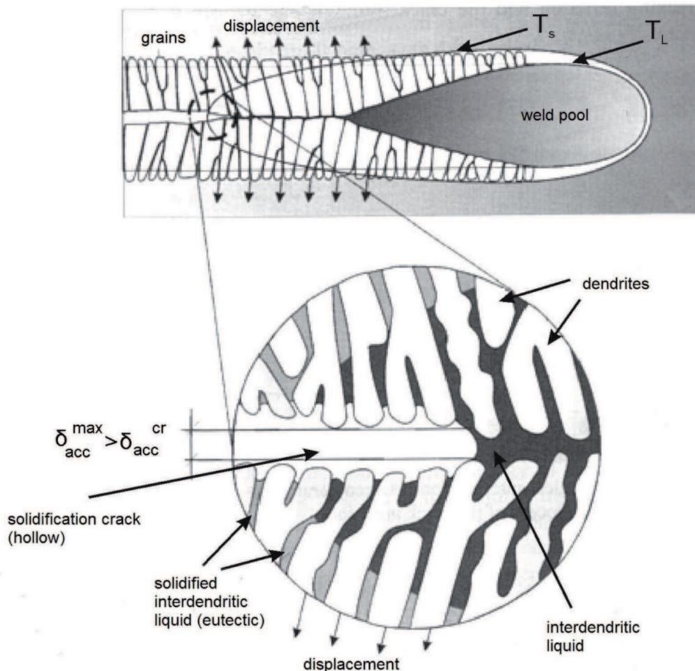
Fig. 3. Mechanism of hot crack formation in a weld;  $\delta_{acc}^{max}$  – maximum interdentritic fluid displacement,  $\delta_{acc}^{cr}$  – critical interdentritic fluid displacement without losing cohesion [6]
