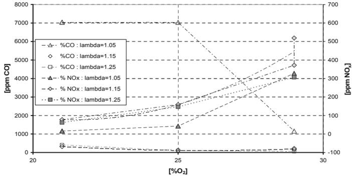
Fig. 5. Effect of oxygen concentration on CO and NO contents for different  $\lambda$  (gas flow of 0.6 m<sup>3</sup>/h)
