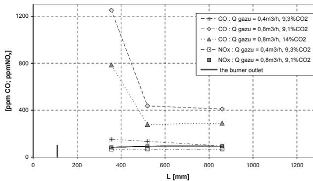
Fig. 3. Variation of CO and NO<sub>x</sub> concentrations along the axis of the chamber for different gas flows (%O<sub>2</sub> = 25 and  $\lambda = 1.25$ )
