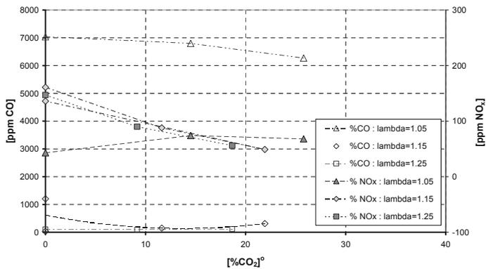
Fig. 7. Effect of CO<sub>2</sub> addition on CO and NO concentrations for 25% O<sub>2</sub> and different  $\lambda$  (gas flow 0.6 m<sup>3</sup>/h)
