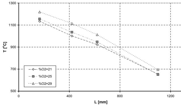
Fig. 1. Temperature drop along the axis of the chamber for different concentrations of oxygen (gas flow = 0.6 m<sup>3</sup>/h and  $\lambda = 1.05$ )
