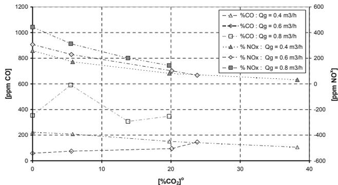
Fig. 11. Effect of CO<sub>2</sub> addition on CO and NO concentration for different gas flows (29% O<sub>2</sub>,  $\lambda = 1.25$ )
