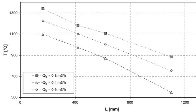
Fig. 2. Temperature drop along the axis of the chamber for different gas flows (%O<sub>2</sub> = 29 and  $\lambda = 1.25$ )
