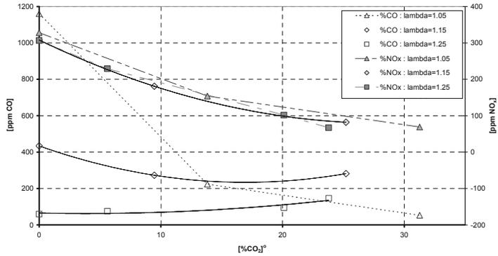
Fig. 8. Effect of CO<sub>2</sub> addition on CO and NO concentrations for 29% O<sub>2</sub> and different  $\lambda$  (gas flow 0.6 m<sup>3</sup>/h)
