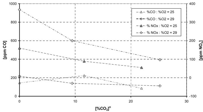
Fig. 9. Effect of CO<sub>2</sub> addition on CO and NO concentrations for different O<sub>2</sub> contents ( $\lambda = 1.15$ , gas flow 0.6 m<sup>3</sup>/h)
