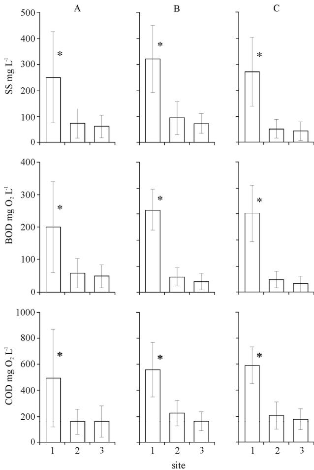
**Fig. 1.** Changes in concentration of SS, BOD<sub>5</sub> and COD (mean ± 1SD, n= 18) on consecutive sites (1 – inlet to AP, 2 – inlet to LP, 3 – outlet from LP, \* indicated significant difference within system, P = 0,05) in three Lemna Systems (A – Falęcin Stary, B – Raków, C – Bąkowiec)
