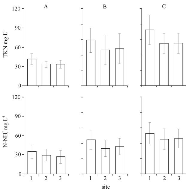
**Fig. 2.** Changes in concentration of TKN and N-NH<sub>4</sub><sup>+</sup> (mean ± 1SD, n= 18) on consecutive sites (1 – inlet to AP, 2 – inlet to LP, 3 – outlet from LP) in three Lemna Systems (A – Falęcin Stary, B – Raków, C – Bąkowiec)
