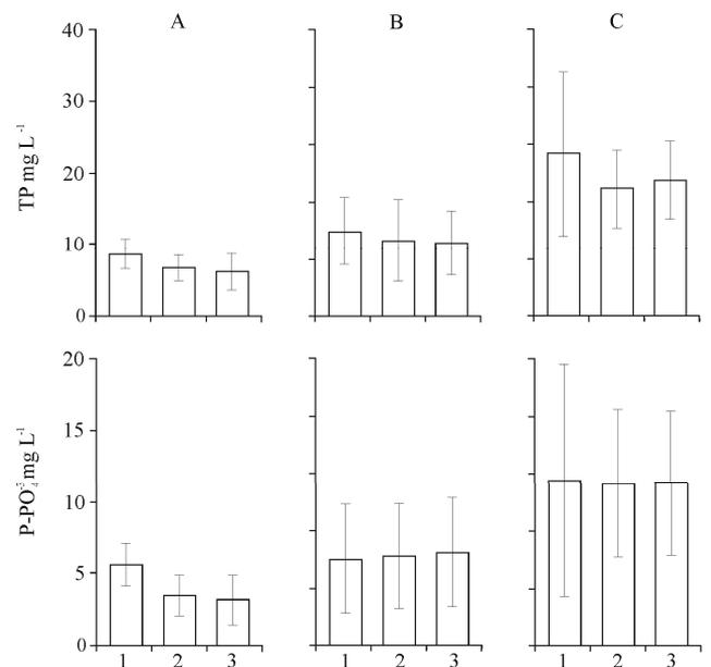
**Fig. 3.** Changes in concentration of TP and P-PO<sub>4</sub><sup>3-</sup> (mean ± 1SD, n= 18) on consecutive sites (1 – inlet to AP, 2 – inlet to LP, 3 – outlet from LP) in three Lemna Systems (A – Falęcin Stary, B – Raków, C – Bąkowiec)
