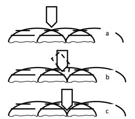
Fig. 7. Different types of incoming bullet-ceramic component contacts: center (a), flank (b) and valley (c)
