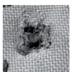
Fig. 5. Front surface of backing with arrested bullet core
