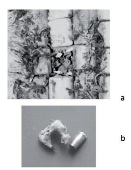
Fig. 6. Typical destruction of ceramic components (a) and bullet (b) (fragments of bullet core and shell)
