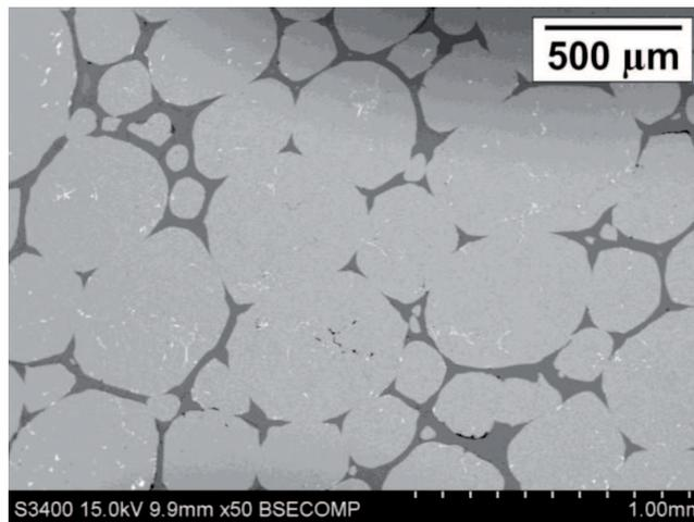
Fig. 4. SEM image (BSE mode) of the AlMg5/Al<sub>2</sub>O<sub>3</sub> composite obtained by pressure infiltration of AlMg5 alloy into Al<sub>2</sub>O<sub>3</sub> foam. Bright area is the metal phase; dark area is the ceramic phase
