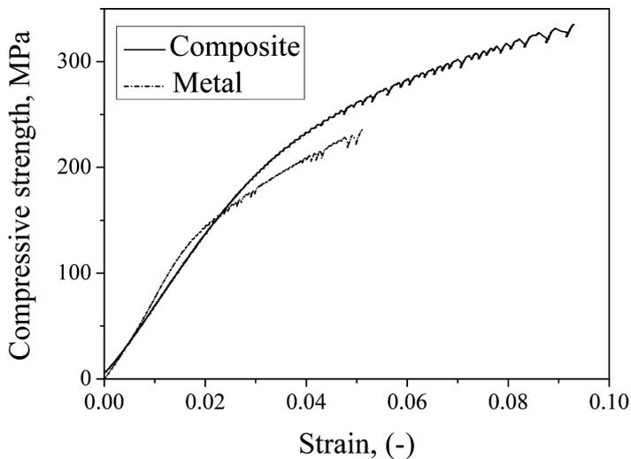
Fig. 6. Stress-strain curve under compressive load for the AlMg5 alloy and the AlMg5/Al<sub>2</sub>O<sub>3</sub> composite
