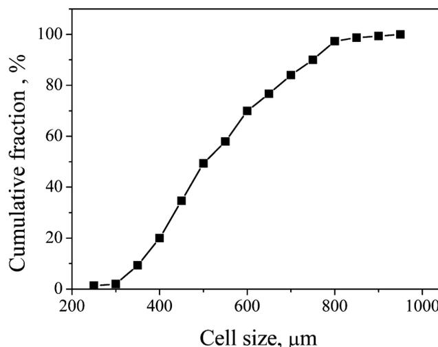
Fig. 2. Cell size distribution of Al<sub>2</sub>O<sub>3</sub> foam measured on the base of image analysis
