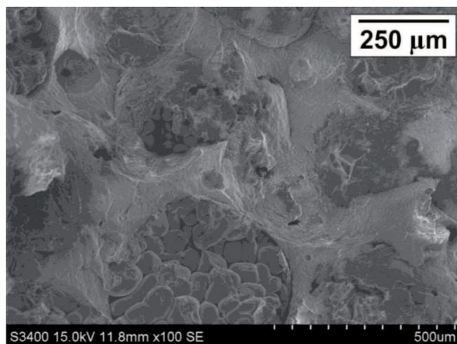
Fig. 5. Fracture section (SEM, SE mode) of the AlMg5/Al<sub>2</sub>O<sub>3</sub> composite obtained by pressure infiltration of AlMg5 alloy into Al<sub>2</sub>O<sub>3</sub> foam. Dark area is the metal phase; bright area is the ceramic phase
