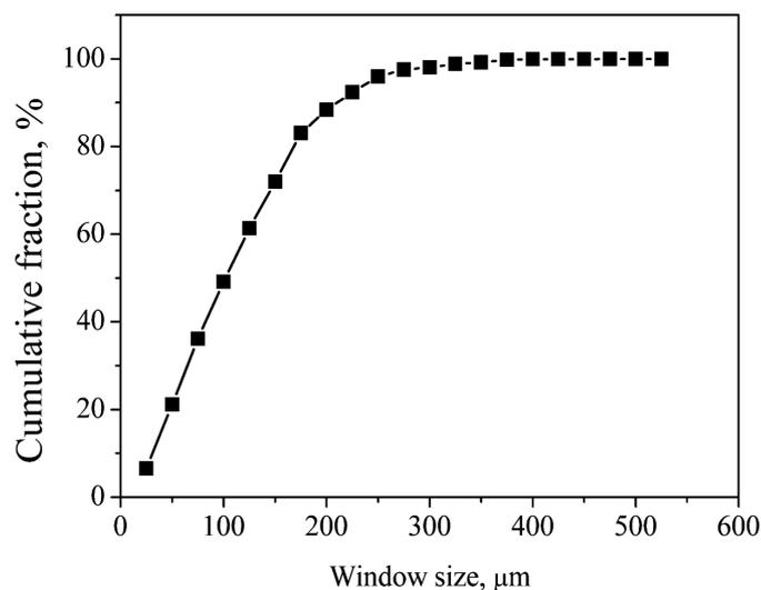
Fig. 3. Window size distribution of the Al<sub>2</sub>O<sub>3</sub> foam measured on the base of image analysis
