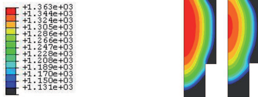
Fig. 4. Temperature field calculated for solidification of the cast steel roll and shown just before – time and slightly after the – time
