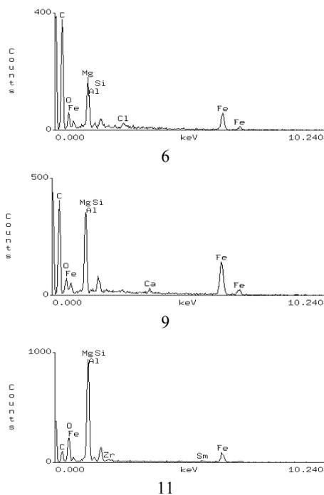
Fig. 7. Scanning photograph of the constituent in the structure of the casting Sample 4 with marked points, in which EDS analysis was performed. Below chosen spectrograms
