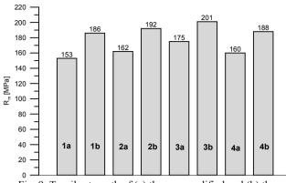
Fig. 9. Tensile strength of (a) the non-modified and (b) the modified AlSi11 alloy cast in: 1) a conventional bentonite-bound mould, 2) an oil-bound sand mould, 3) a die, 4) a shell mould (phenol-formaldehyde resin binder)
