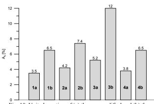
Fig. 10. Unit elongation of (a) the non-modified and (b) the modified AlSi11 alloy cast in: 1) a conventional bentonite-bound mould, 2) an oil-bound sand mould, 3) a die, 4) a shell mould (phenol-formaldehyde resin binder)
