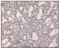
Fig. 5. Structures of AlSi11 alloy without modification (die)
