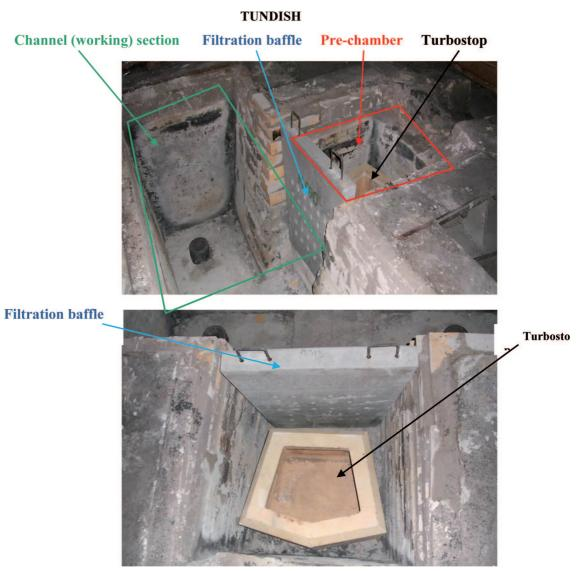
Fig. 5. Tundish filter – option II
