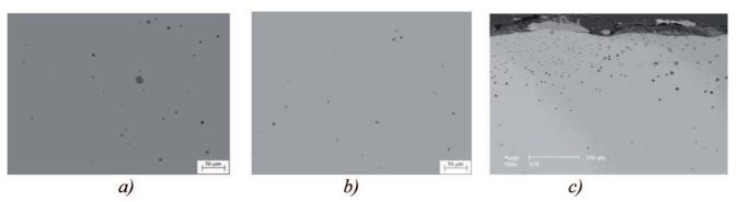
Fig. 3. Non-metallic inclusions in sample of non-filtered steel (a), steel filtered through corundum filter (b), and steel solidified in filter channel, close to the metal – ceramic material interphase boundary (c)
