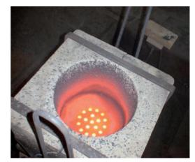
Fig. 7. Hot top with filter following completed casting process
