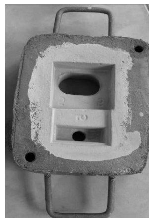
Fig. 2. View of sand mould with plate of austenitic steel (1) placed in its cavity: a – bottom half of mould, b – top half of mould
