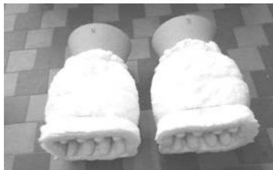
Fig. 3. Moulds with insulation ready for tests
