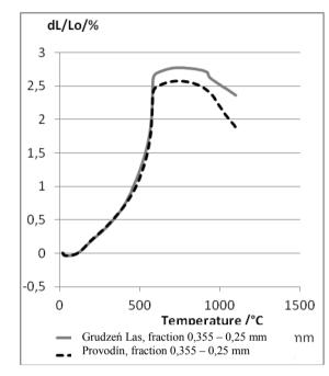
Fig. 2. Thermal expansion of silica sand
