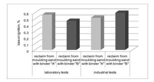
Fig. 16. Loss on ignitron in reclaim moulding sands with binders from the laboratory and industrial production
