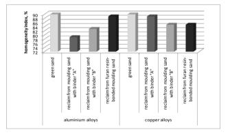
Fig. 6. Homogeneity index in the reclaim moulding sand poured aluminum and copper alloys
