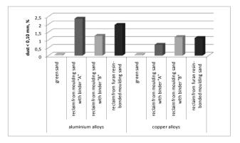
Fig. 7. Dust in the reclaim moulding sand poured aluminum and copper alloys
