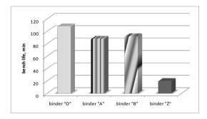
Fig. 1. Bench life of moulding sands with studies types of soluble sodium silicate and furan resin
