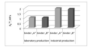
Fig. 10. Bending strength of moulding sand with binders from laboratory and industrial production
