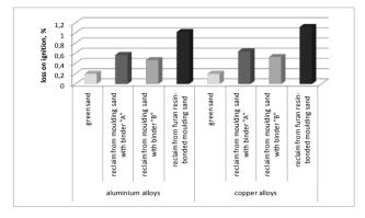
Fig. 8. Loss on ignitron in the reclaim moulding sand poured aluminum and copper alloys
