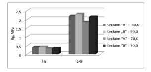
Fig. 19. Bending strength of moulding sands with a variable participation of the reclaim from the industrial reclamation test
