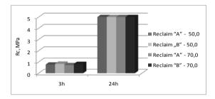
Fig. 18. Compressive strength of moulding sands with a variable participation of the reclaim from the industrial reclamation test
