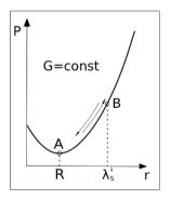
Fig. 2. A parabola of the entropy production for the eutectic rodlike structure formation [5, 6]
