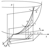
Fig. 1. A paraboloid of the entropy production drawn in function of two thermodynamic forces  $(X_c, X_r)$ , with the added so-called "technological" coordinate system  $(v, \lambda)$  [5, 6]
