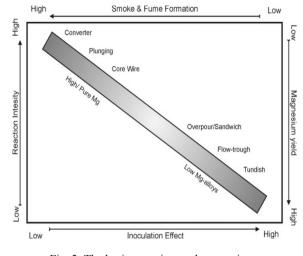
Fig. 2. The basic overview and comparison of spheroidization methods
