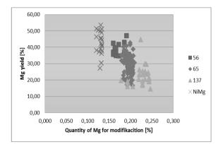
Fig. 5. Mg yield and Mg<sub>us</sub> for necessary the final content Mg<sub>res</sub> in the range (0.040 to 0.060) [%]
