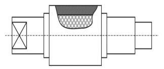
Fig. 1. Sketch of two-layer roll, view shell layer (purple) and the core layer (green-white)
