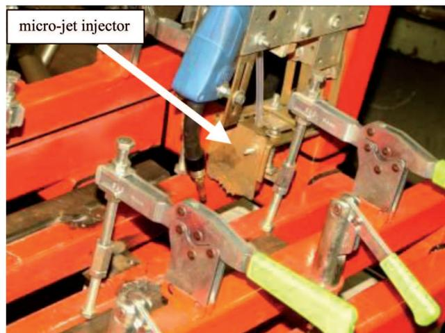
Fig. 4. Equipment for MIG welding with micro-jet injector
