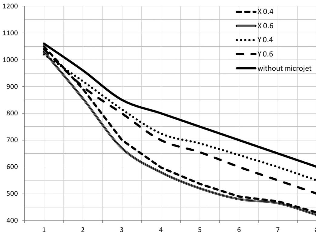
Fig. 5. Weld cooling conditions with micro-jet injector
