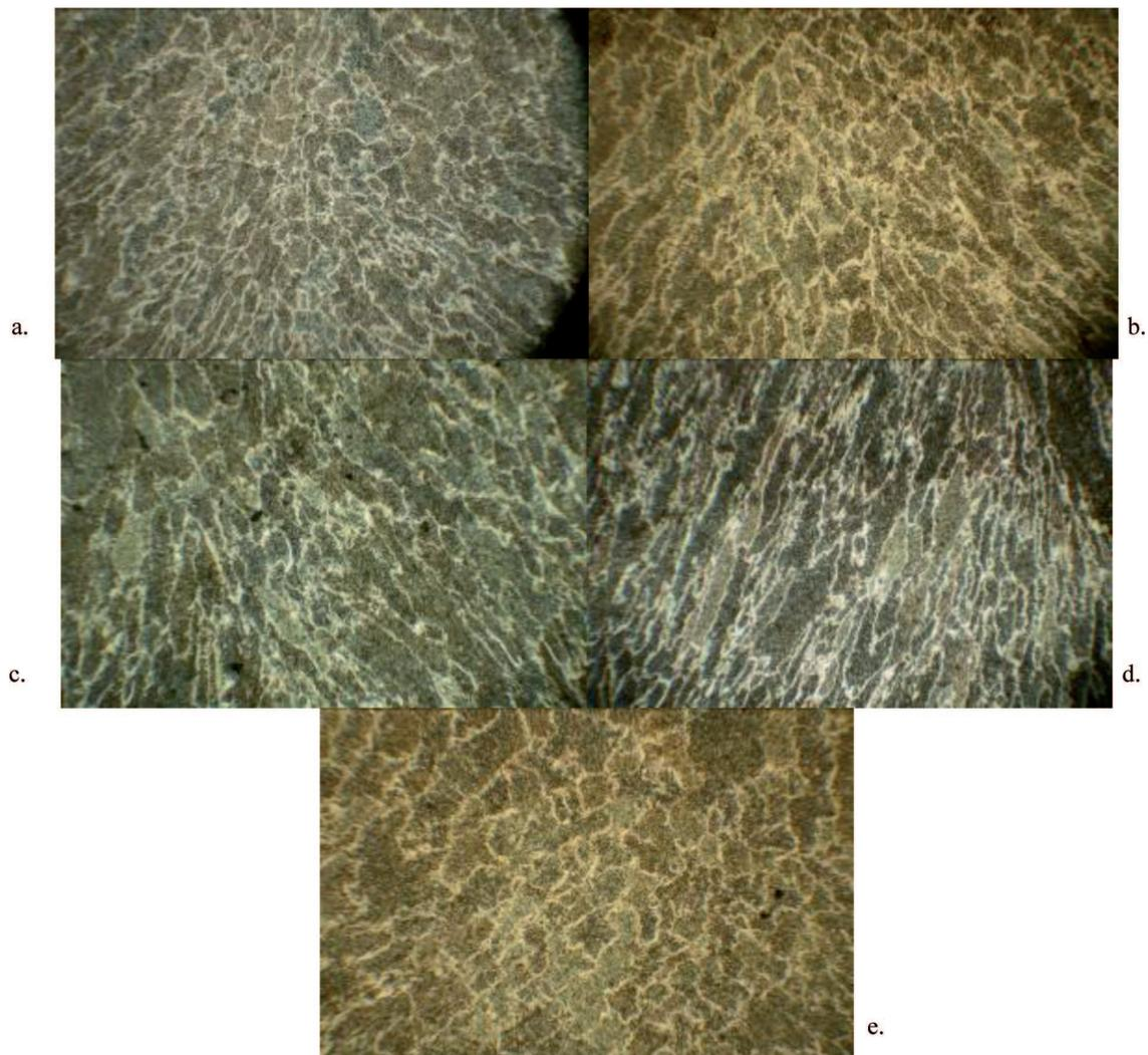
Fig. 6. Example of typical analyzed structures for MIG: a) standard MIG; b) MIG with micro-jet (X 0.4); c) MIG with micro-jet (X 0.6); d) MIG with micro-jet (Y 0.4); e) MIG with micro-jet (Y 0.6). Magnification x 30
