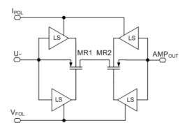
Fig. 4. Simplified scheme of the AMP1 resistive feedback.
