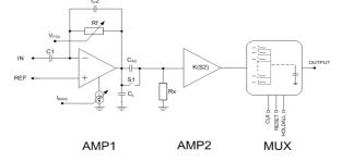
Fig. 2. Simplified block diagram of single readout channel.
