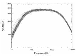
Fig. 6. Distribution of the gain for  $V_{FOL}$ = -0.2V.
