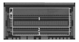
Fig. 1. Photo of the 64-channel chip where: 1 - AMP1, 2 - AMP2, 3 - analogue multiplexer, 4 - voltage references.
