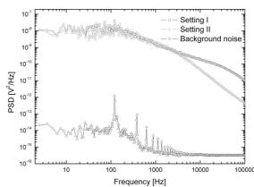
Fig. 9. Power spectral density of output noise of ASIC for two different pass-band settings and instrumentation noise.
