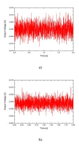
Fig. 10. Typical output reffered noise of the channel for diffrent pass-band settings: a) Setting I, b) Setting II.
