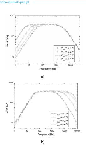
Fig. 5. Frequency response of single channel: a) low cut-off frequency tuning, b) high cut-off frequency tunning.
