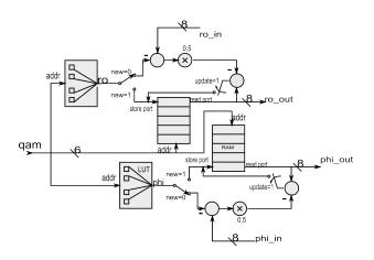
Fig. 10. Simplified diagram of the inner structure of a DP device.
