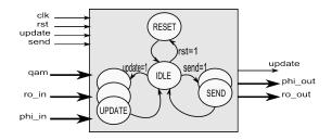
Fig. 11. Simplified block diagram of a predistorter device together with the FSM diagram.
