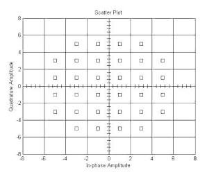
Fig. 1. Rectangular QAM constellation 32QAM. Values of  $a_n^I$  and  $a_n^Q$  are not normalized but are set to simple integers instead.
