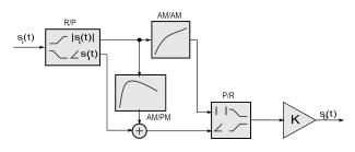
Fig. 2. Memoryless behavioral model of power amplifier.
