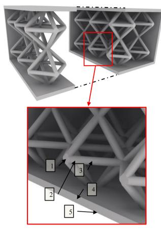
Fig. 2. Specified regions of microstructure investigation; 1 – node; 2 – near node cross-section; 3 – cross-section between the nodes; 4 – cross-section of closing wall; 5 – outside surface of closing wall
