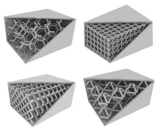
Fig. 1. Internal topologies of skeleton castings developed in Foundry Department
