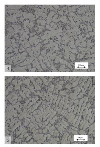
Fig. 3. AlSi11 alloy structure: 1 – node; 2 – near node crosssection; 3- cross-section between the nodes; 4- cross-section of closing wall; 5 – outside surface of closing wall
