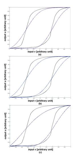
Fig. 5. Major hysteresis loop obtained experimentally (black-colored line) and the loop calculated using the probability density functions: a) Gauss-Gauss for parameters  $N = 1, \sigma = 0.582933, Ho = 0.425094$ ; b) lognormal-gaussian for  $N = 1, \sigma = 0.601153, Ho = 0.454492$ ; c) factorized-Lorentzian for  $N = 1, \sigma = 0.614152, Ho = 0.427471$ .
