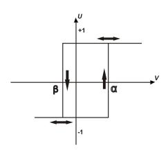
Fig. 2. The relay defined by a pair of threshold values  $(\beta, \alpha)$ . The output of the relay is +1, when the input is greater than  $\alpha$ , -1 when the input is smaller than  $\beta$  and stays unaltered when the input stays in the  $(\beta, \alpha)$  range.
