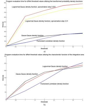
Fig. 8. Program evaluation time dependence on increasing value of threshold using a) three transformed probability density functions; b) characteristic function of integration area. Black color marks the Gauss-Gauss density function, blue - Lorentz density function and red marks the lognormalgaussian density function.
