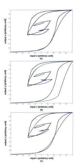
Fig. 7. The minor hysteresis loop obtained experimentally (black-colored line) and a loop obtained using the probability density functions (blue-colored line): a) Gauss-Gauss for parameters  $N = 1, \sigma = 0.582933, Ho =$ 0.425094; b) lorentzian for  $N~=~1, \sigma~=~0.614152, Ho~=~0.427471;$ c) lognormal-gaussian for  $N = 1, \sigma = 0.601153, Ho = 0.454492$ . The calculations were made using the characteristic function of the integration area.
