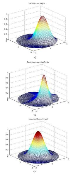
Fig. 4. An example of probability density functions, achieved for  $\sigma = 1$  and  $H_0 = 1$ . a) Gauss-Gauss density function; b) Factorized-Lorentzian density function; c) Lognormal-gauss density function.
