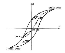
Various magnetisation curves (major and minor loops) presented Fig. 1. for an unspecified ferromagnetic material. The major hysteresis loop on the plane (H, B) is obtained by changing the value of the coerced magnetic field H from the value  $-H_{max}$  to  $H_{max}$  and vice versa. There can be also be observed the phenomenon of the minor loop closure  $(H_1, B_1) \rightarrow (H_2, B_2)$ .
