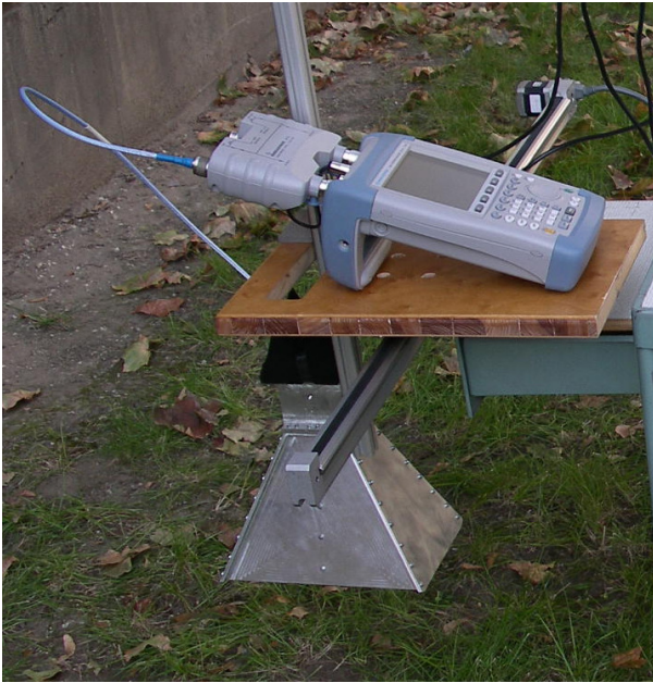
Fig. 2. Mobile GPR Setup with R&S FSH-6 in outdoor measurement.
