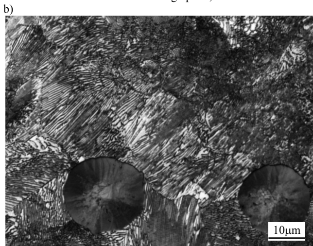
b) microstructure: nodular graphite, pearlite
