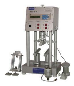
Fig. 7. The stand for bending tests [14]
