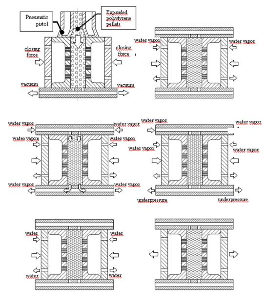
Fig. 1. The diagram of polystyrene patterns making
