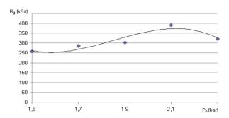
Fig. 10. Dependence of the resistance to bending  $R_g$  in the option of the passing steam pressure  $P_p$ ,  $R_g=f(P_p)$
