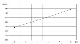
Fig.11. The influence of the time of the passing the water steam through the pattern on its resistance to bending at constant pressure which was  $P_p = 2.1$  bar and constant autoclave parameters which were  $t_A = 7$  s and  $P_A = 1.7$  bar
