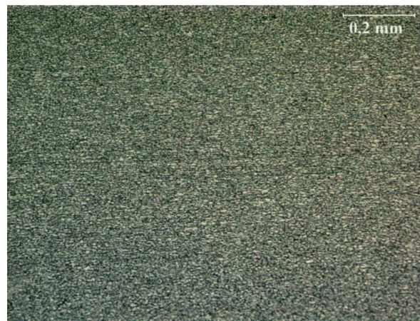
Fig. 10. Microstructure of DP600 base material; magn. 100x, etched with 5-% nital, light microscope
