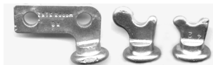
Fig. 5. Castings made in the low permeability ceramic mould
