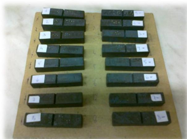
Fig. 1. Test specimens and 1.2343 Dievar
