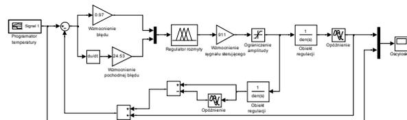
Fig. 4. Diagram of the resistance furnace control with fuzzy controller and Smith predictor
