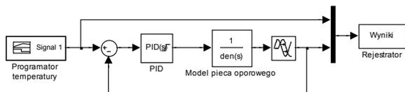
Fig. 2. Modeled in MATLAB / Simulink resistance furnace control system with PID controller
