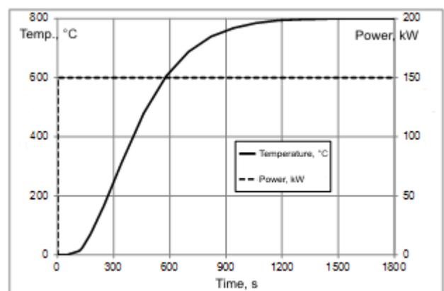
Fig. 1. Graph temperature changes in the resistance foundry furnace chamber when you turn on the maximum power supply
