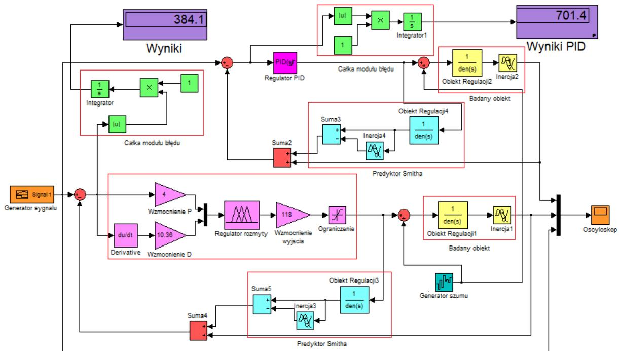
Fig. 6. Scheme designed in Simulink system simulation to compare the control quality criterion K, calculated according to equation (2), for the system with PID controller and fuzzy controller for the assumed internal structure
