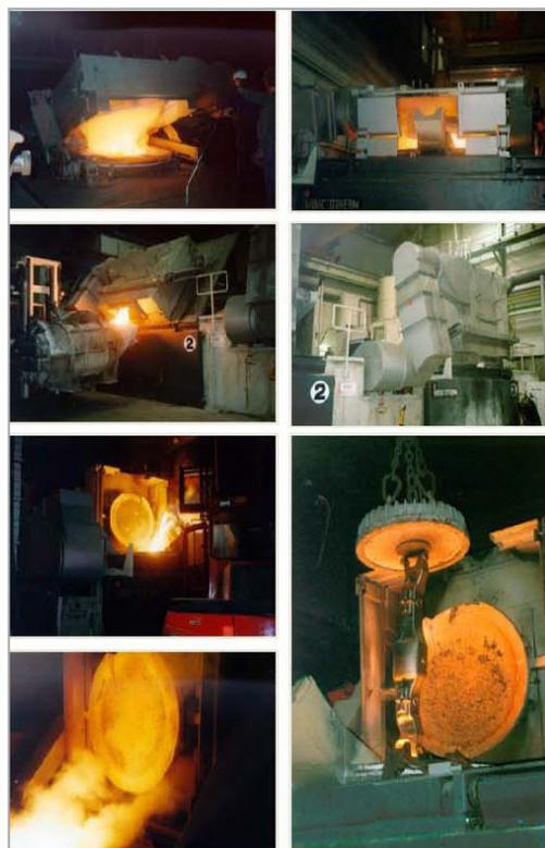
Fig. 2. Suction hood for induction furnace
