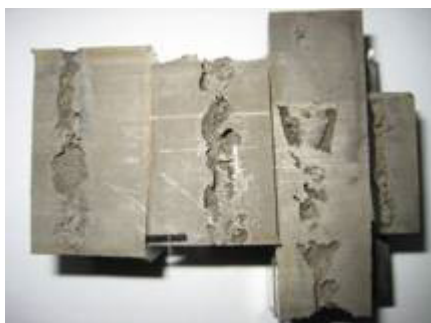
Fig. 3. Axial section of the IN-713C nickel alloy master heat ingot. Samples taken from these sections weighing about 1.2 kg were remelted in a Balzers VSG-02 induction furnace with an \text{Al}_2\text{O}_3 crucible in which, owing to the stability of technological parameters, high purity materials were produced. Melting was conducted in a vacuum of about 10^{-3} . Before pouring of moulds, the working space of the furnace was flushed with argon. Pouring was carried out in an argon atmosphere at a pressure of about 900hPa.
