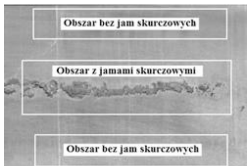
Fig. 7. Areas in master heat ingots where samples were taken for the ATD thermal analysis
