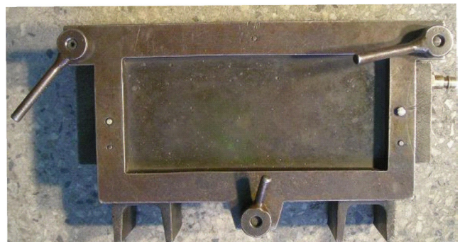
Fig. 10. Horizontal experimental core-box of a capacity 0.816 dm^3 (the background mosaic is not seen)
