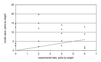
Fig. 6. Comparison of the distribution of data generated by the network and the experimental data, input data - compactability
