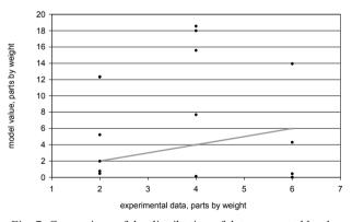
Fig. 7. Comparison of the distribution of data generated by the network and the experimental data (test data), input data: compressive strength, compactability, permeability
