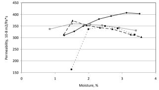
Fig. 2. The influence of water content on permeability for the moulding sands with different active bentonite content
