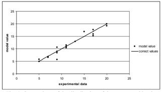
Fig. 4. Comparison of the distribution of data generated by the network and the experimental data (test data set), input data: compressive strength, compactability, permeability. output data: non-active binder, the network model: MLP 3-8-1, model quality: 0,9683 [12]
