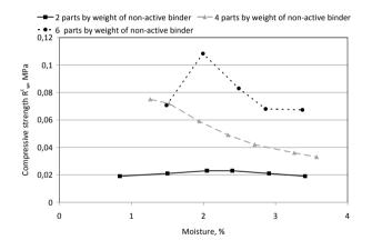
Fig. 1. The influence of water content on compressive strength R<sub>c</sub><sup>w</sup>, for the moulding sands with different active bentonite content
