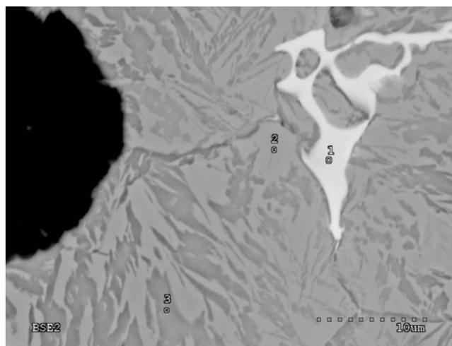
Fig. 6. The microstructure of nodular cast iron with carbides and upper bainite and measurement points of chemical composition
