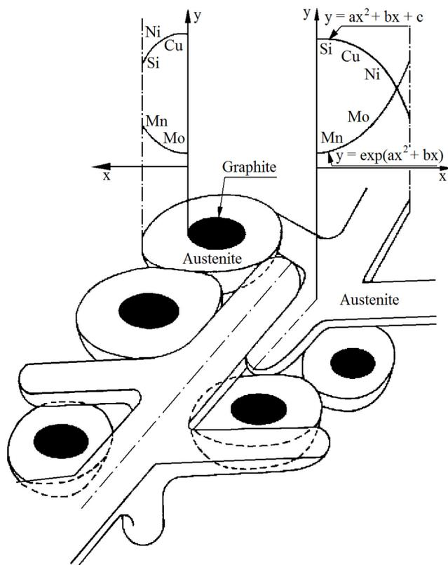
Fig. 1. The scheme of nodular cast iron structure and microsegregation of its elements [4]
