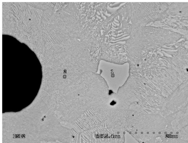
Fig. 4. Microstructure of pearlitic nodular cast iron with carbides with a measurement points of chemical composition
