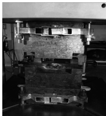
Fig. 2. A set of tools for die forging on a 2.5MN press – disassembled
