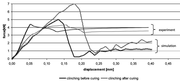
Fig. 8. Simulated separation force evolution in the pull test - comparison between: clinching before curing and clinching after curing
