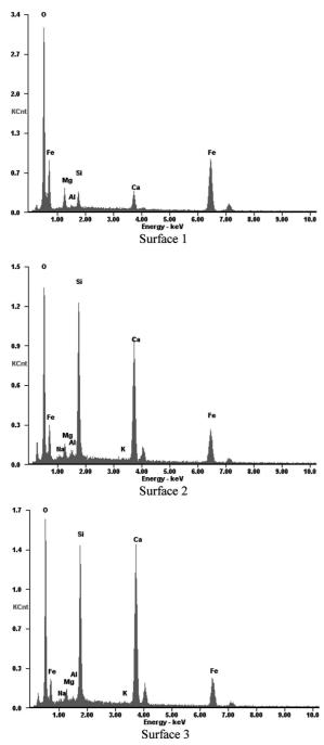
Fig. 3. EDX spectrum of surface 1, 2, 3
