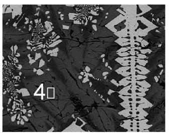
No.4b Fig. 4. Microstructure of the sinter
