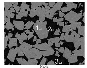
Fig. 2. Microstructure of the sinter
