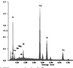
Fig. 8. EDX spectrum of surface No.7b
