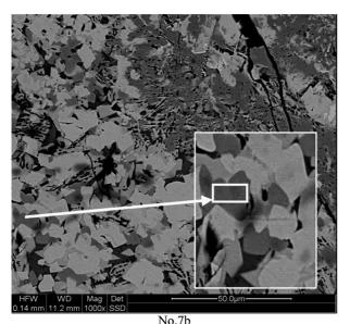
Fig. 7. Microstructure of sinter – samples
