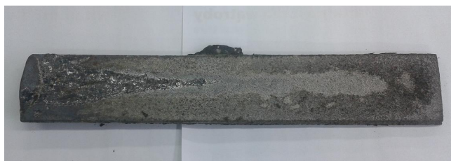
Fig. 7. Casting after being knocked-out – from the side of shaped samples without protective coatings
