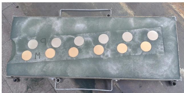
Fig. 6. View of the mould from the side of shaped samples with two kinds of protective coatings (marking: M – coating 1, P – coating 2)
