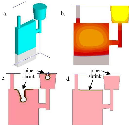
Fig. 6. Influence of critical value of solid fraction in database (NovaFlow&Solid – NFS CV): a – 3D geometry with bottom chill, b – location of hotspot, c – both  $f_{s,crit}=0,2$  (total shrink 1,5%), d – both  $f_{s,crit}=0,7$  (total shrink 4,9%)
