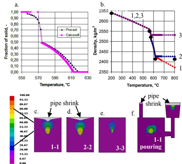
Fig. 7. The  $f_s=f(T)$  (a) and  $\rho=f(T)$  (b) applied to CS and Procast macro models tests –  $\rho$  variations for Procast: 1-1, 2-2 and 3-3 and for CS between the black points (• – •). Examples of shrinkage positions for 3 cases  $\rho=f(T)$  (c, d, e). Procast for critical piping solid fraction CPSF=0,3, critical macroporosity solid fraction CMSF=0,7, f – shrinkage position (with pouring).
