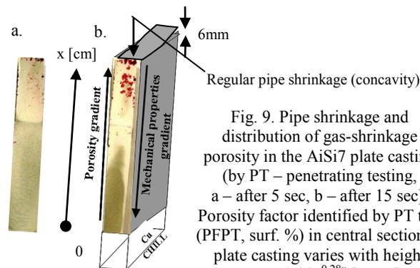
Fig. 9. Pipe shrinkage and distribution of gas-shrinkage porosity in the AlSi7 plate casting (by PT – penetrating testing, a – after 5 sec, b – after 15 sec). Porosity factor identified by PT test (PFPT, surf. %) in central section of plate casting varies with height PFPT=0,88e<sup>0,28x</sup> [x, cm].
