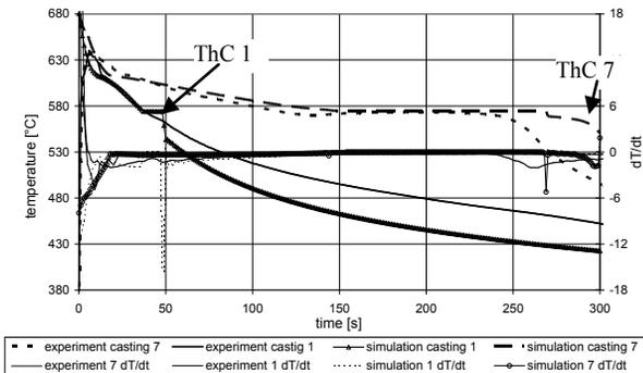
Fig. 5. Results of the real and simulated experiment –  $T=f(t)$  and  $dT/dt=f'(t)$  as the best conformity to the thermal macro-model (for chosen two thermocouples positions. Local solidification time TC 1: 49sec (exp&sim) and TC 7: 264 sec (exp) & 269 sec (sim).
