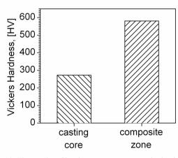
Fig. 10. The results of hardness measurements obtained for M0 alloy
