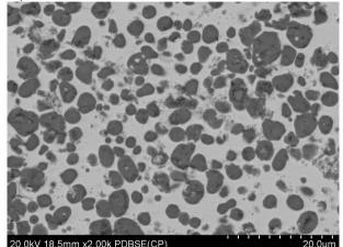
Fig. 3. BSE image of the composite zone in M0 alloy
