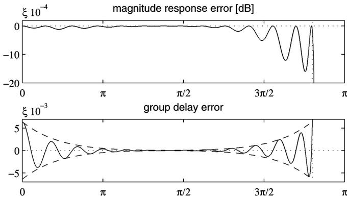
Fig. 6. FD filter of length  $N = 53$  with  $\omega_a = 0.9\pi$  and  $\varepsilon = -0.25$  designed with weighted magnitude of group delay error used as the error function. Dashed lines present group delay error limits resulting from weighting function.
