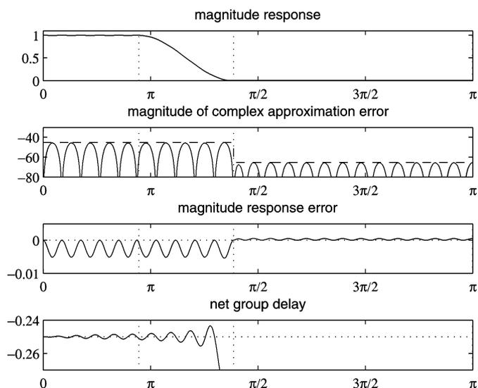
Fig. 8. RC filter of length  $N = 94$ ,  $L = 3$ ,  $\alpha = 0.33$  and  $\varepsilon = -0.25$  with fullband optimization. Filter designed with weighted magnitude of complex approximation error used as the error function. Dashed lines represent error limits resulting from weighting function.
