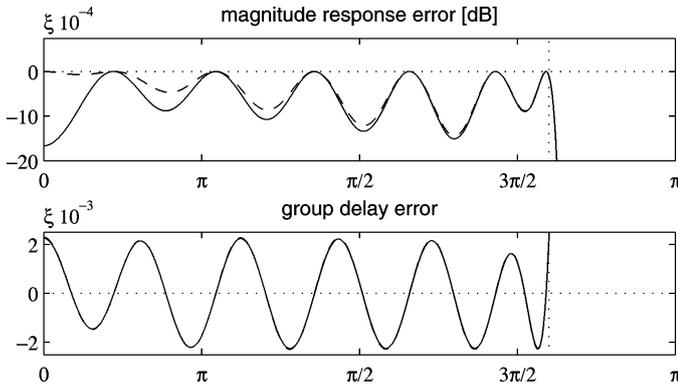
Fig. 1. Filter of the length  $N = 25$  with  $f_a = 0.4$  and  $\varepsilon = -0.25$  with minimized magnitude response error. The case with zero order condition at  $f = 0$  – dashed line and with first order condition at  $f = 0$  – solid line.
