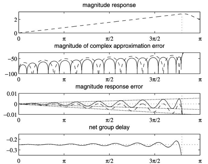
Fig. 7. Differentiators of length  $N = 33$  with  $\omega_a = 0.9\pi$  and  $\varepsilon = -0.25$  designed with weighted magnitude response error used as the error function. Solid lines – the case with only zero order conditions ( $i_k = 0$ ) and dashed lines – the case with zero and first order conditions ( $i_k = 0, 1$ ).
