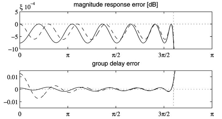
Fig. 2. Filter of the length  $N = 25$  with  $\omega_a = 0.8\pi$  and  $\varepsilon = -0.25$  with minimized group delay error. The case with zero order condition at  $f = 0$  – dashed line and with first order condition at  $f = 0$  – solid line.
