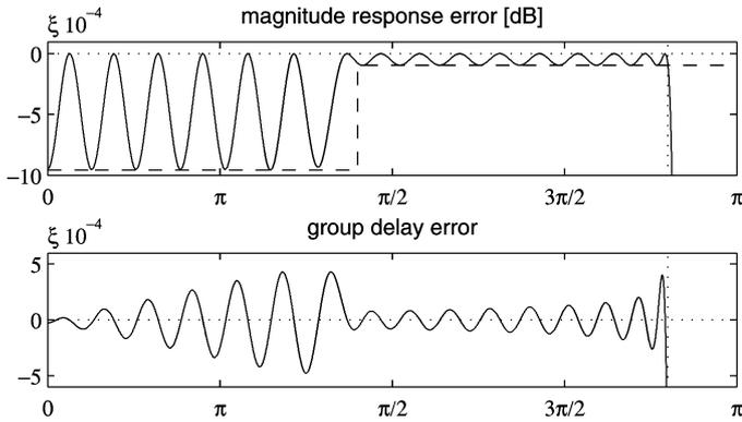
Fig. 5. FD filter of length  $N = 64$  with  $\omega_a = 0.9\pi$  and  $\varepsilon = 0.25$  designed with weighted magnitude response error used as the error function. Dashed lines present group delay error limits resulting from weighting function.
