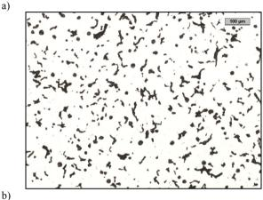
Fig. 1. Microstructure of castings with wall thickness of 5 mm: (a) heat No. I, (b) heat No. IV
