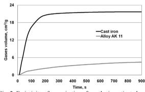
Fig. 2. Emissivity of gases in time, from the investigated sands: after pouring the mould with alloy AK 11 of a temperature of 700°C (grey line); after pouring the mould with cast iron of a temperature of 1350°C (black line)
