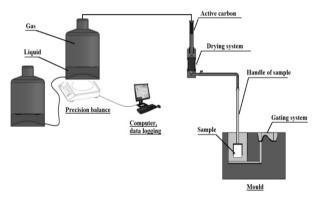
Fig. 1. Experimental stand for the determination of the emitted gases volume and the BTEX emission [1]
