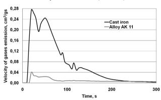
Fig. 3. Velocity of gases emission, from the investigated sands: after pouring the mould with alloy AK 11 of a temperature of 700°C (grey line); after pouring the mould with cast iron of a temperature of 1350°C (black line)
