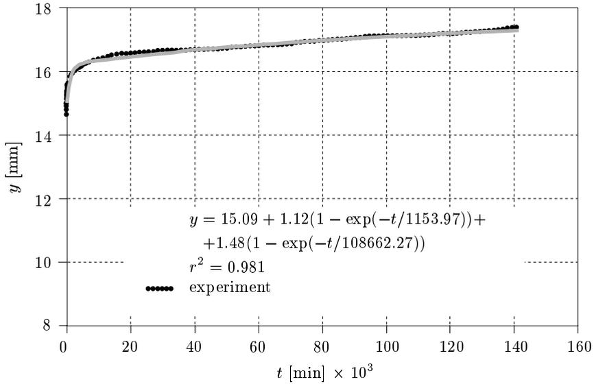
Fig. 5. Total deflection of composite I-beam – creep data fitted by 5-parameter equation (3)
