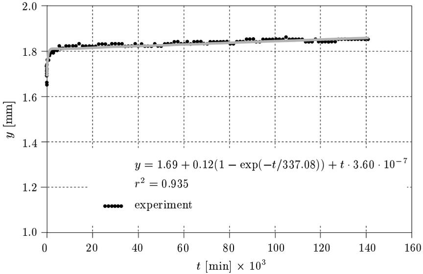
Fig. 7. “Pure” deflection of composite I-beam – creep data fitted by 4-parameter equation (2)
