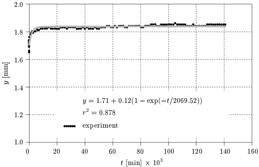
Fig. 6. “Pure” deflection of composite I-beam – creep data fitted by 3-parameter equation (1)
