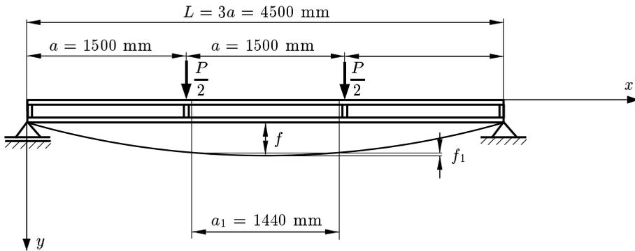
Fig. 3. Diagram of the composite I-beam load and deflections measurement
