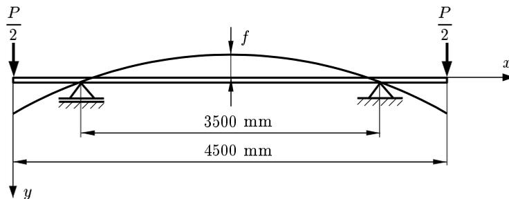
Fig. 2. Diagram of the flange load and deflection measurement
