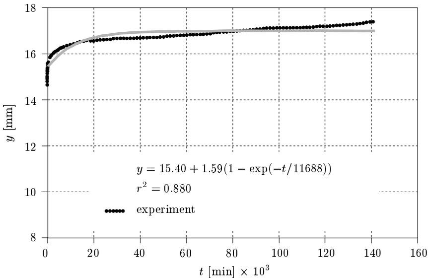
Fig. 4. Total deflection of composite I-beam – creep data fitted by 3-parameter equation (1)
