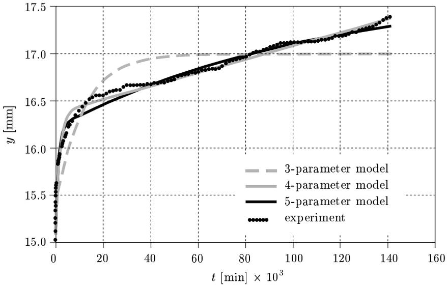
Fig. 8. Total deflection of composite I-beam – quality of fitting to the creep data by varied creep models within the zone of delayed, viscoelastic deformations
