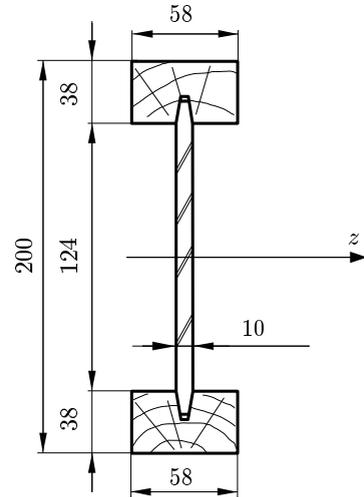
Fig. 1. Cross-section dimensions of the composite I-beam [mm]
