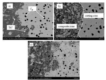
Fig. 5. BSE images of microstructures obtained in a transition region between the composite zone and the casting core in castings M100 (a), M90 (b) and M50 (c)
