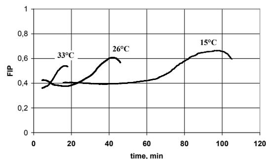
Fig. 3. Variability of the FIP index in time for the same furan sand in ambient temperatures of 15, 26 and 33°C (laboratory chamber, thermostated)
