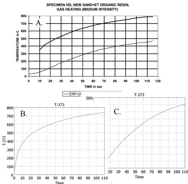
Fig. 6. Comparison of experimentally determined temperatures (A) and simulation results (COMSOL Multiphysics) of thermal balance of the HD Plus® sample heated with the gas flame (B and C) as a result of a positive validation of the thermal parameters (substitute heat conductivity, heat capacity)
