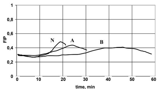
Fig. 4. Variability of the FIP index in time for the furan sands for three different sand matrices (A – mechanical, B – thermal, N – new sand) and for the same set of binder 1% + „slow” hardener 0,4%, ambient temperature approx. 22°C
