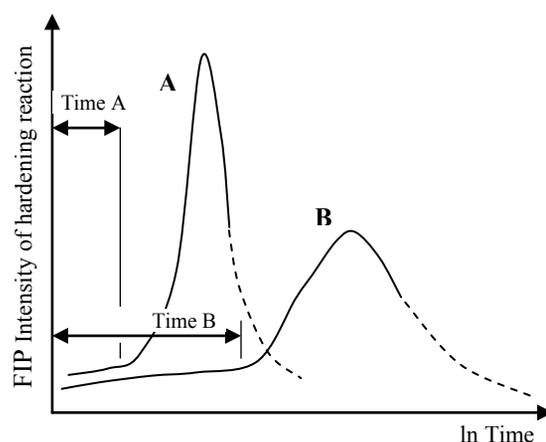
Fig. 1. Scheme of the extreme variability of kinetics of the molding sand hardening reaction (surface layers): A. sufficient life time and relatively quick hardening reaction (Time A – acceptable molding time), B. too low life time and too slow binding (Time B – unfoundedly long acceptable molding time)
